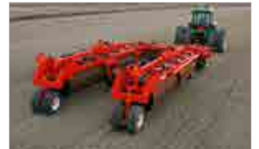
The forward unfolding system goes from transport mode to field mode in minutes.
