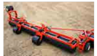
The shorter drum sections float independently, ensuring you roll every inch of your land evenly.
