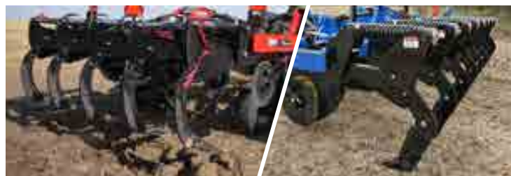
PARABOLIC SHANKS WITH HYDRAULIC TRIP
