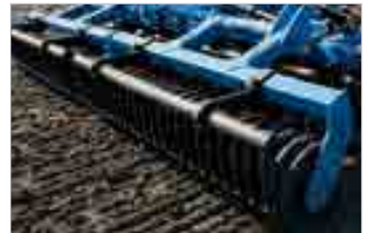
RUBBER ROLLERS WITH HD SCRAPERS
