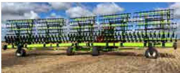
The steerable wing wheels allow the DHX to easily go in or out of transport mode.
