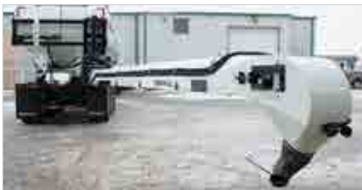
SIDE MOUNTED CONVEYOR
